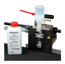
6. Ensure that there is sufficient lubricant in the lubrication device, see Section 9.3.2.1
