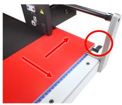
10. Place the workpiece on the precision circular table saw and push it against the stops.
