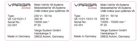
Figure 3 Motor unit plates 230 V~ mains voltage
