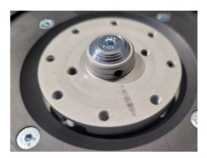
11. Remove the mount from the motor shaft with the help of the pull-off tool.
