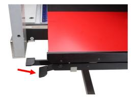
9. If necessary, set the scale for the right stop 2. To do this, operate the lever to raise the right stop 2.
