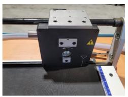
5. Remove the two screws (front VA 10 = M6x20) (front VA 11 / front VA 21-15 / front VA 31-15 = M8x22) from the guide rod.
