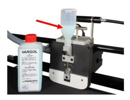
6. Ensure that there is sufficient lubricant in the lubrication device, see Section 9.3.2.1
