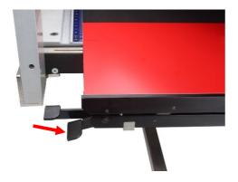
9. If necessary, set the scale for the right stop 2. To do this, operate the lever to raise the right stop 2.
