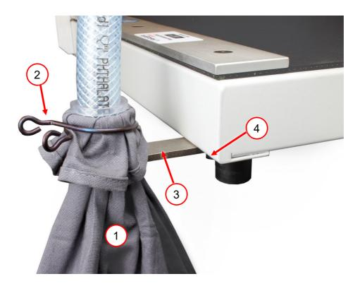
Figure 21 Fitting the VARGA VA 10 chip bag
