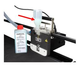
6. Ensure that there is sufficient lubricant in the lubrication device, see Section 9.3.2.1
