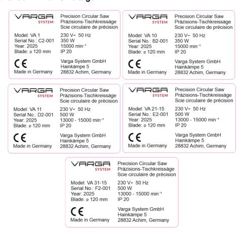
Figure 2 Machine type plates 230 V~ mains voltage
