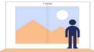
WE SUGGEST A 1" OVERLAP WHEN USING THE OPAQUE VERSIONS. DO NOT TRY TO SPLIT CUT AND BUTT THE OVERLAP WHEN USING THE OPAQUE MATERIAL, IT CAN LEAVE A WHITE LINE. IT IS OK TO SPLIT CUT THE OVER-LAP ON THE NON-OPAQUE VERSIONS. BE CAREFUL USING TAPE TO ALIGN THE MATERIAL WITH LATEX INKS. REMOVING IT TOO FAST CAN PULL THE INK OFF.
